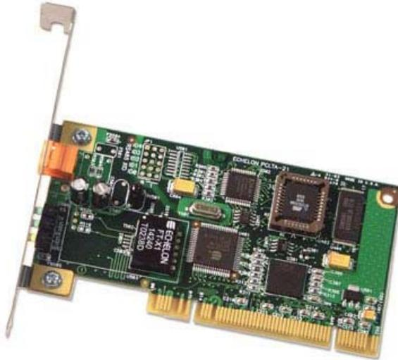
The PCLTA-21 card Model 74504 (TP-RS485) includes jumpers that must be configured to set the correct speed on the RS-485 channel.
