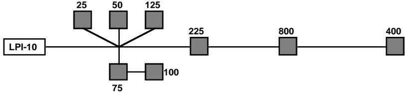
Simplification Step Three and equivalent network for power specifications:
