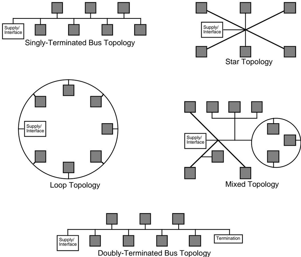
**Figure 1.2** Typical Wiring Topologies Supported By the Link Power System
