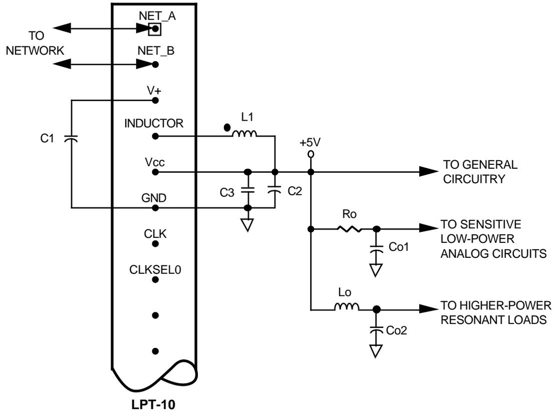
Figure 4.1 Post-Filtering of Vcc
