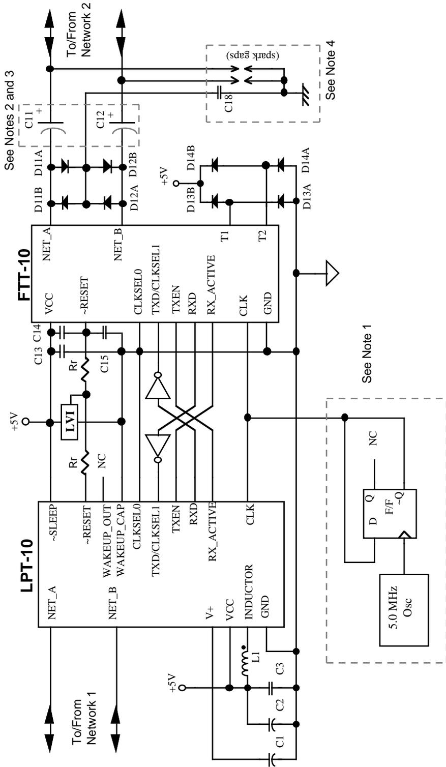
Figure 2.5 Two-Way Repeater Schematic
