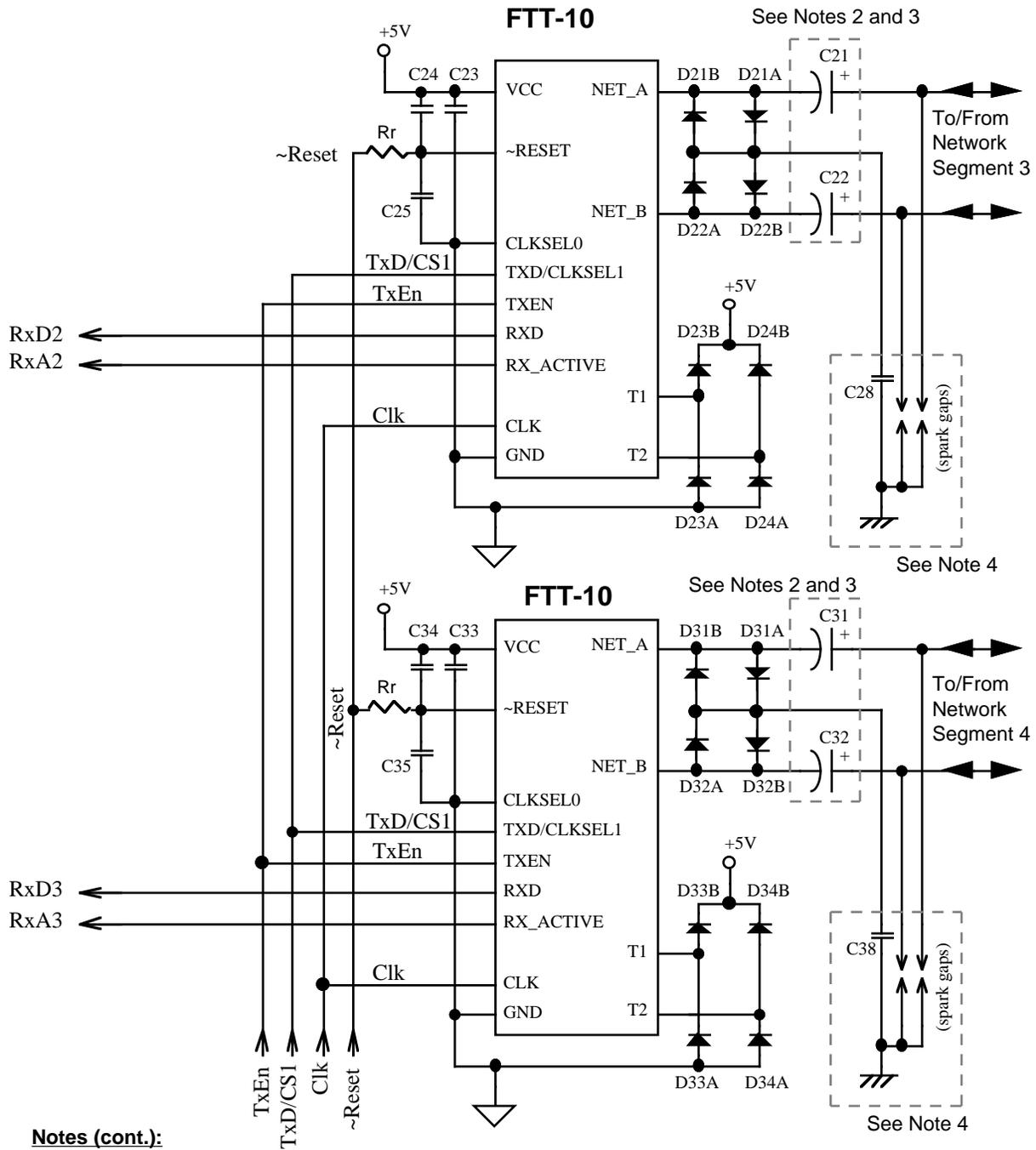
**Figure 2.6b** Four-Way Repeater Schematic (page 2 of 2)
