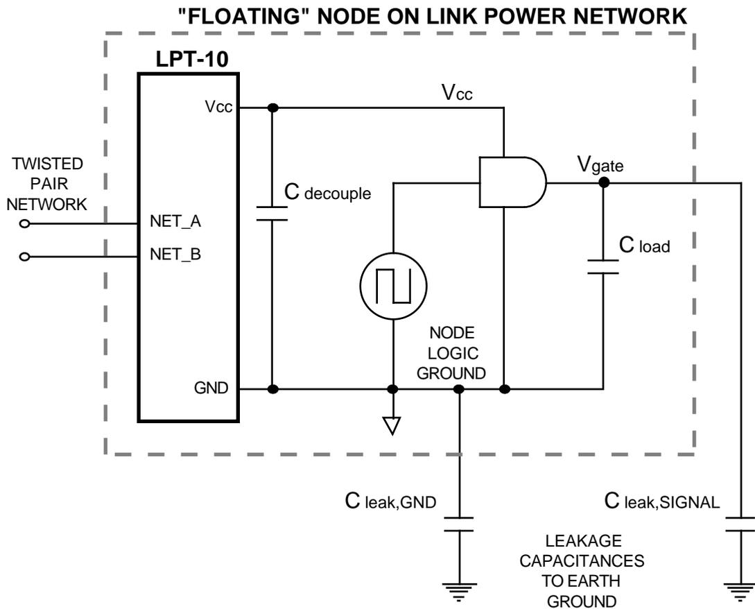
**Figure 6.1** Parasitic Leakage Capacitances to Earth Ground
