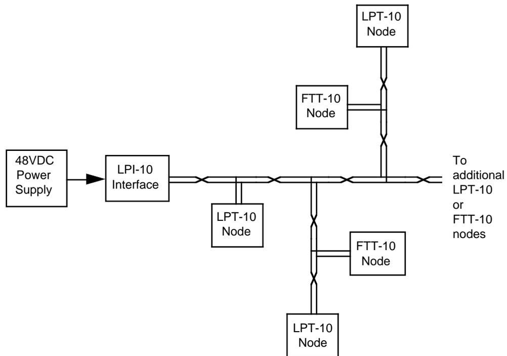
**Figure 1.1** Free Topology Link Power System
