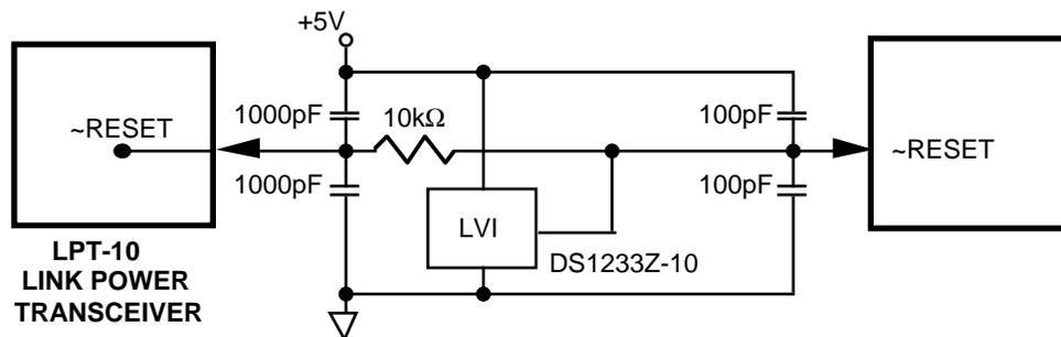
Figure 2.2 LPT-10 Transceiver -- Alternate Reset Circuit
