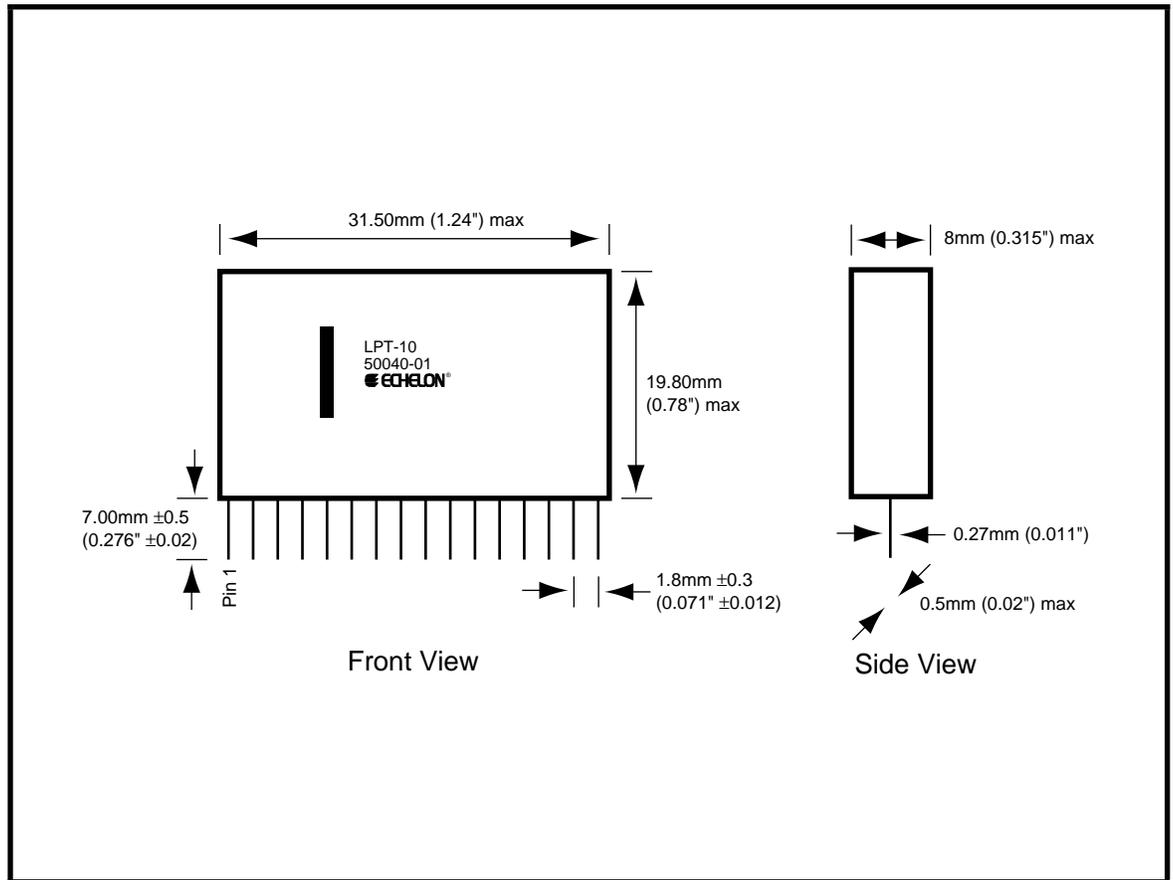
**Figure 3.1** LPT-10 Transceiver Mechanical Footprint
