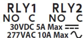
The relay contacts support up to 277VAC @ 10A or 30VDC @ 5A
