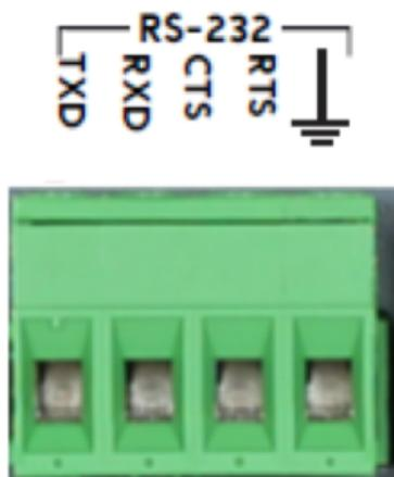
The screw terminals on the RS-232 plugs accept 0.22mm – 3.3mm (22 – 12AWG) gauge solid wire. The optimum tightening torque for the screw terminals is 0.75 Newton-meters (6 lbs. in.) maximum. The ideal flathead screwdriver
