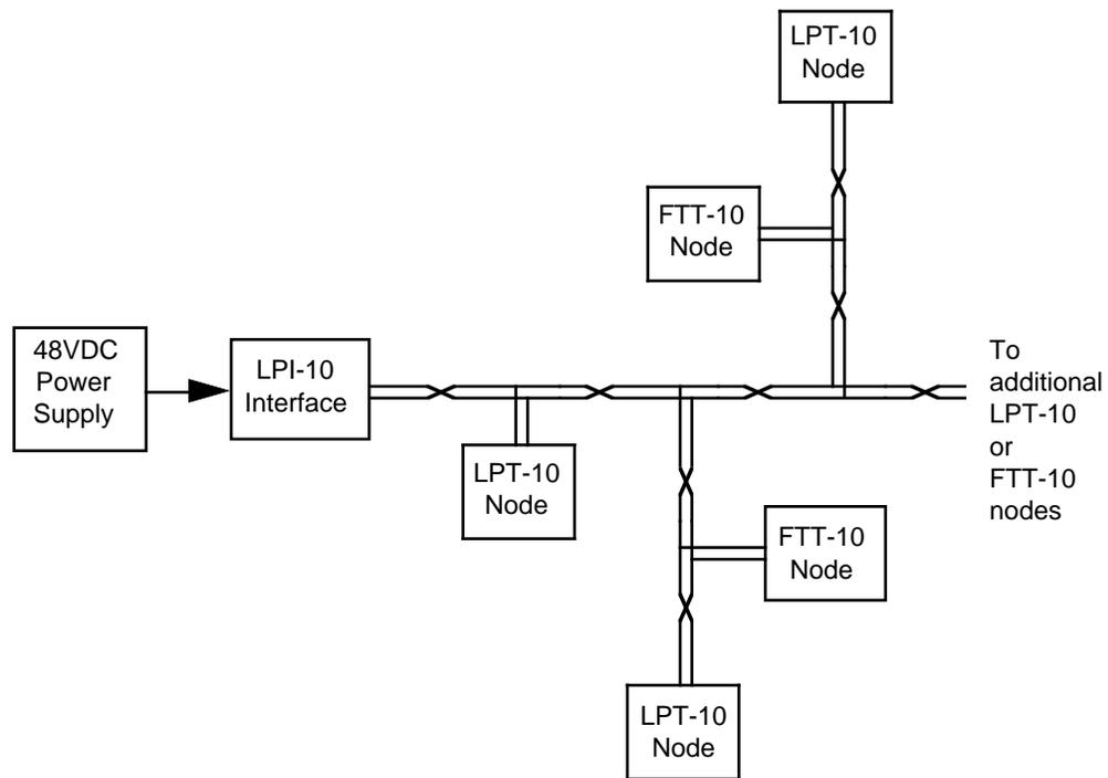
**Figure 1.1** Free Topology Link Power System
