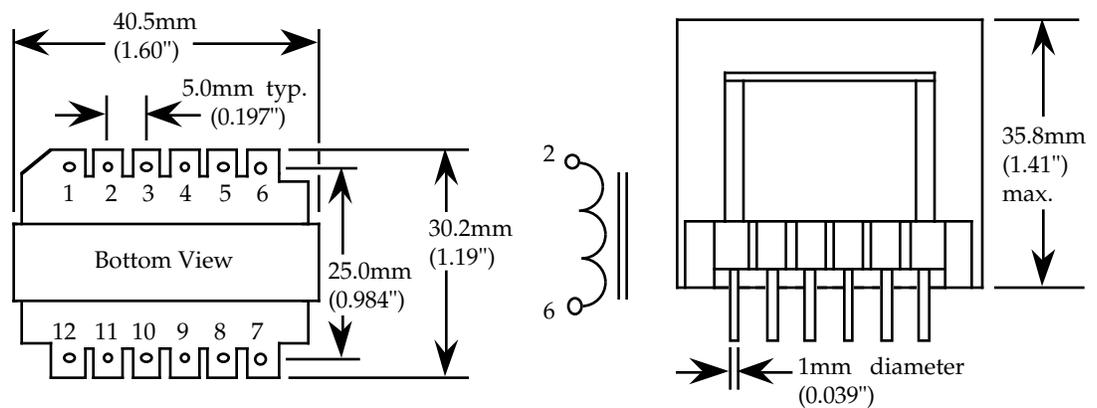
**Figure A.5** Mechanical Dimensions for Inductor (Recipe "A")
