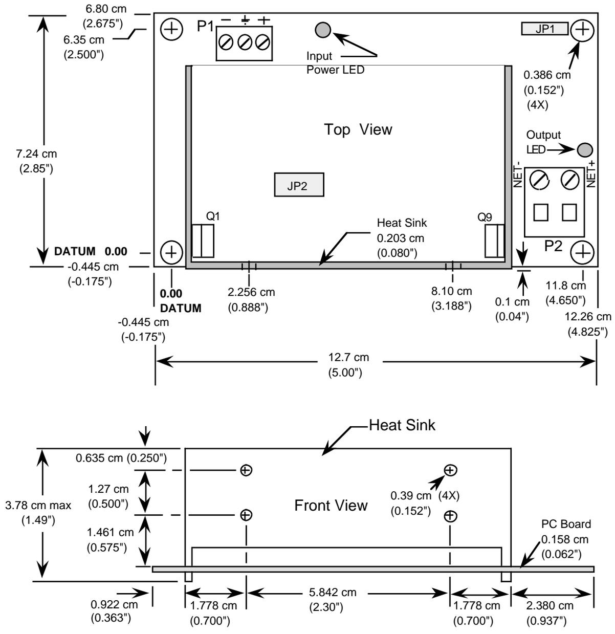
Figure 3.1 LPI-10 Module Dimensions
