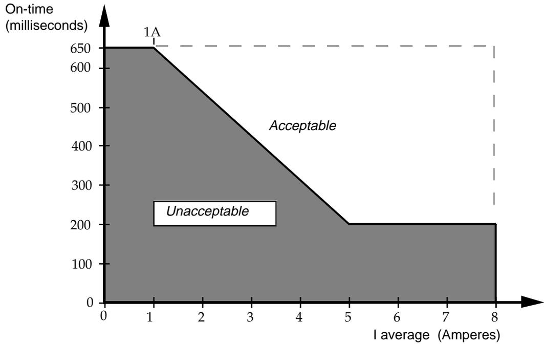
**Figure A.3** Power Supply Startup Interval Behavior
