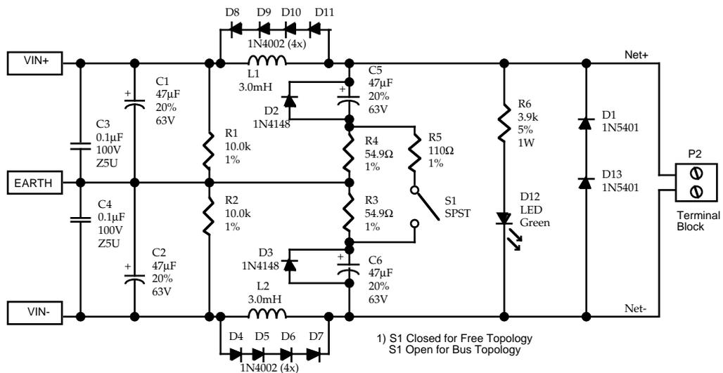
**Figure A.4** Echelon Passive Coupler Schematic
