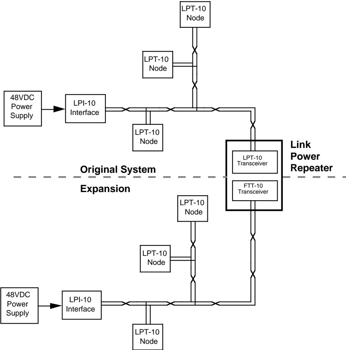
**Figure 1.3** Link Power Repeater for System Expansion
