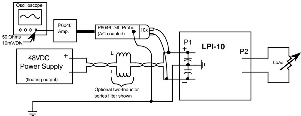
**Figure 2.3** Differential Noise Measurement
