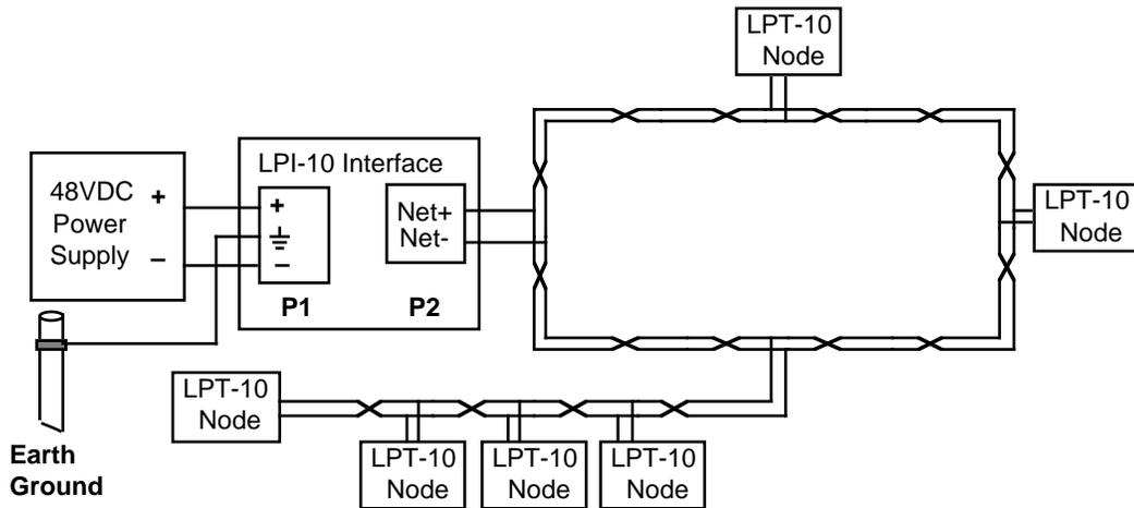
**Figure 2.1** LPI-10 Module Interconnections
