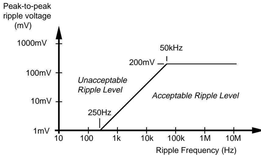
**Figure A.2** Power Supply Output Ripple Voltage Requirement
