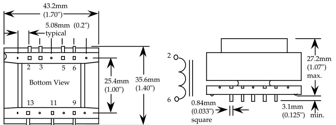
**Figure A.6** Mechanical Dimensions for Inductor (Recipe "B")
